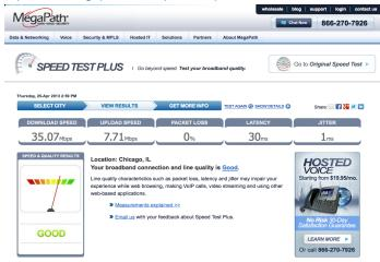
Comprehensive VoIP readiness test. This example shown was performed when a particular connection was busy with a lot of other Internet traffic, causing excessing jitter. IP-Audio would work if more buffering at each receive end is dialed-in.
