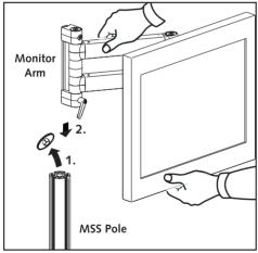
Do not forget to assemble the **Security Set** onto the Pole **first!** It comes with every Monitor Arm (#YT3230) and every Fleximount (#YT3231). You will need a **Pole Desktop Mounting Kit** (#YT3245) to mount the MSS Pole onto the desktop. The PDM-Kit contains an M10x70 screw, two washers and two cable clamps. Screw the Monitor Arm's (Fleximount's) **VESA Attachment** and the TFT Monitor before mounting the Monitor Arm (Fleximount) onto the MSS Pole.
