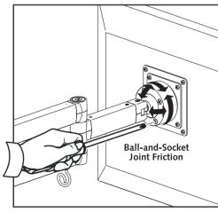
Set the monitor's height by loosening and tightening the Quick-Release Ratchet. The friction of the Height Slider can be adjusted by loosening and tightening the upper screw. The Articulated Joints enable to position the monitor horizontally, the viewing distance in particular. You may softly freeze the monitor's inclination by adjusting the friction of the Ball-and-Socket-Joint.
