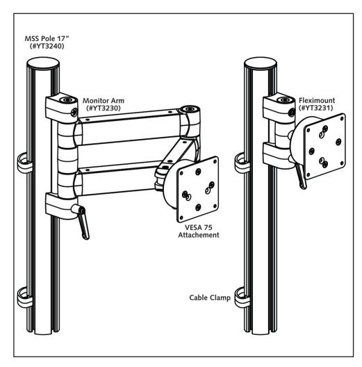
Each **Fleximount** (#YT3231) can hold monitors weighing up to 12kg (26lbs) and each **Monitor Arm** (#YT3230) up to 10kg (22lbs). You can mount up to four monitors at the same height on a single **MSS Pole**. It is available in three standard lengths: MSS Pole 17" (#YT3240), MSS Pole 21" (#YT3243) and MSS Pole 33" (#YT3241). The Cable Clamps are part of the **Pole Desktop Mounting Kit** (#YT3245).
