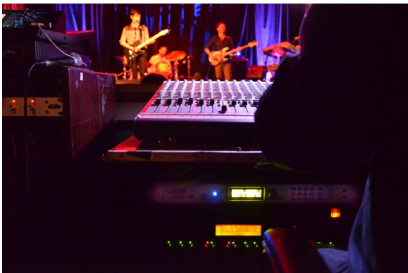
Nashville, Tennessee's 3rd & Lindsley concert venue sends a live performance to a local radio station via broadband, using the Telos Z/IP ONE codec beneath the console.
