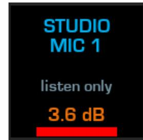
In case Full Control of a Source which is currently loaded onto a different console is desired, the source must be unloaded so that its control is released by its current owner.
