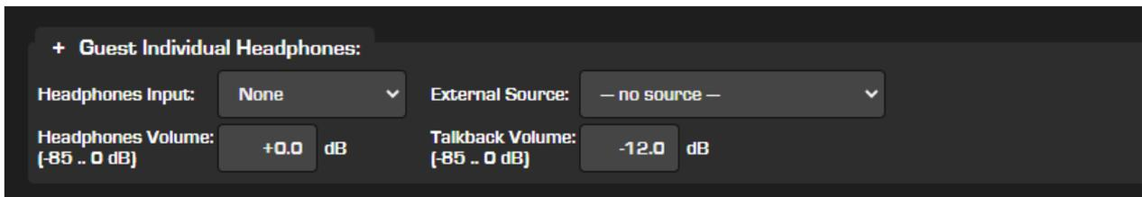
**Note** - In this case, if there is an Accessory module associated to this source, this will be able to control the **Headphones Input** and **Headphones Volume** parameters. This is the place where the Accessory module settings are stored, within a Show.
