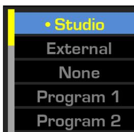
Push the encoder to display the Headphone Input source list. Scroll the list and push the encoder knob to select the desired source and return to the volume control screen.
