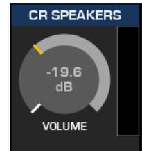
A white start detent can be located either at the beginning (left edge) of the circular background, or in the middle, according to the nature of the associated parameter (example: *pan* will have a center detent, while *gain* will have a left detent). In case the function, or parameter, associated with a Gauge is turned off, the Gauge will reflect this by changing the color of the indicator, and the text.
