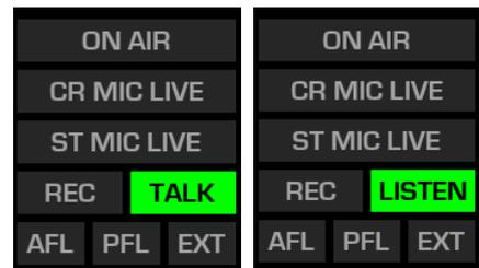
Both these actions will enable the Talkback function, turning the corresponding signal on in the MTS Home screen.
