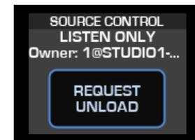
Pushing the **REQUEST UNLOAD** button will make a confirmation message appear on the screen. If **OK** is selected, and if the channel which currently owns it, is turned OFF, then the Source will be unloaded and control released to the requesting channel.
