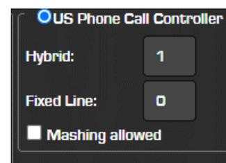
The final step is to define how you want to handle mix-minus. Quasar (and all Axia consoles) automatically generates mix-minus (N-1, or "clean feed") for each phone caller taken to air.
