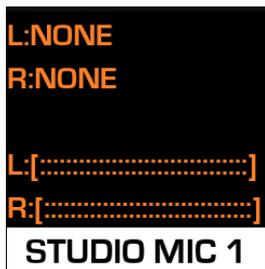
Upon touching the knob, two volume level bars for the selected feed will be displayed. The Volume level, and Source selection, can be adjusted independently for the Left and Right channels.
