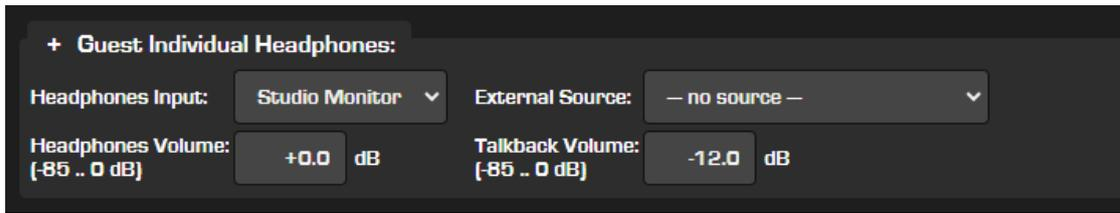
The **External Source** drop-down menu contains all those sources that were configured as “External” by selecting the corresponding flag in the Source Availability section. They correspond to those available on the module when the **EXT** key is pressed.
