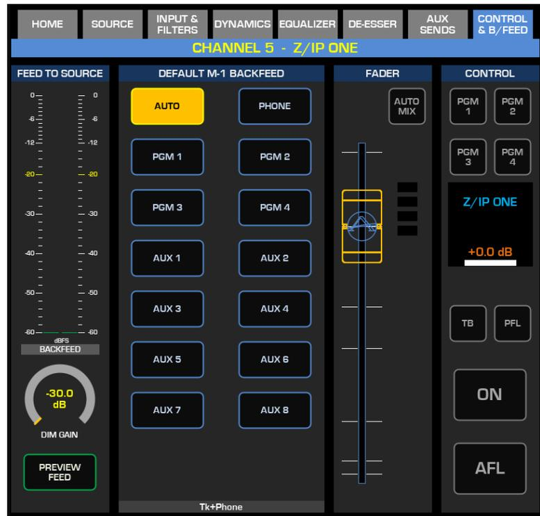
The **CUSTOM BACKFEED selector** is displayed only in case the Source type is a Microphone, a Codec or a Phone and the Backfeed is set as Custom type. It provides:
