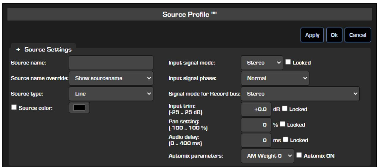
In the **Source Settings** section, select **Operator Microphone** from the **Source type** drop-down list. In the **Source name** field, type a useful name, like “Host” or “Board Op”, that the DJ can easily identify. This is the name that will be shown on the display of fader strip the source is loaded to.
