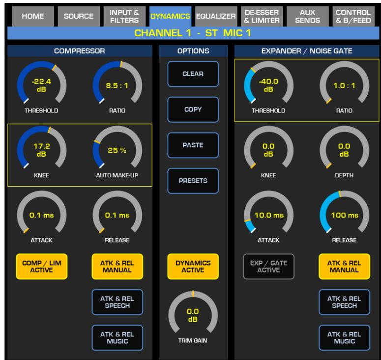
The EXPANDER / NOISE GATE section provides:
