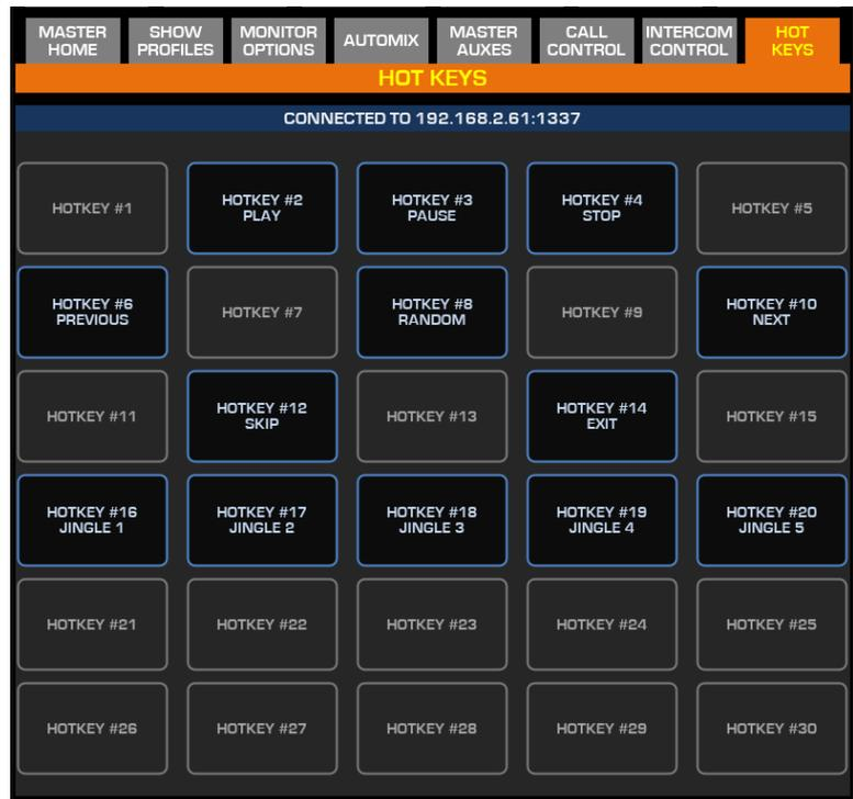
30 user-programmable on-screen buttons can send a control string to any device connected over a TCP link, providing that the IP address and Port # of the receiving ends are entered into the console Web UI.
