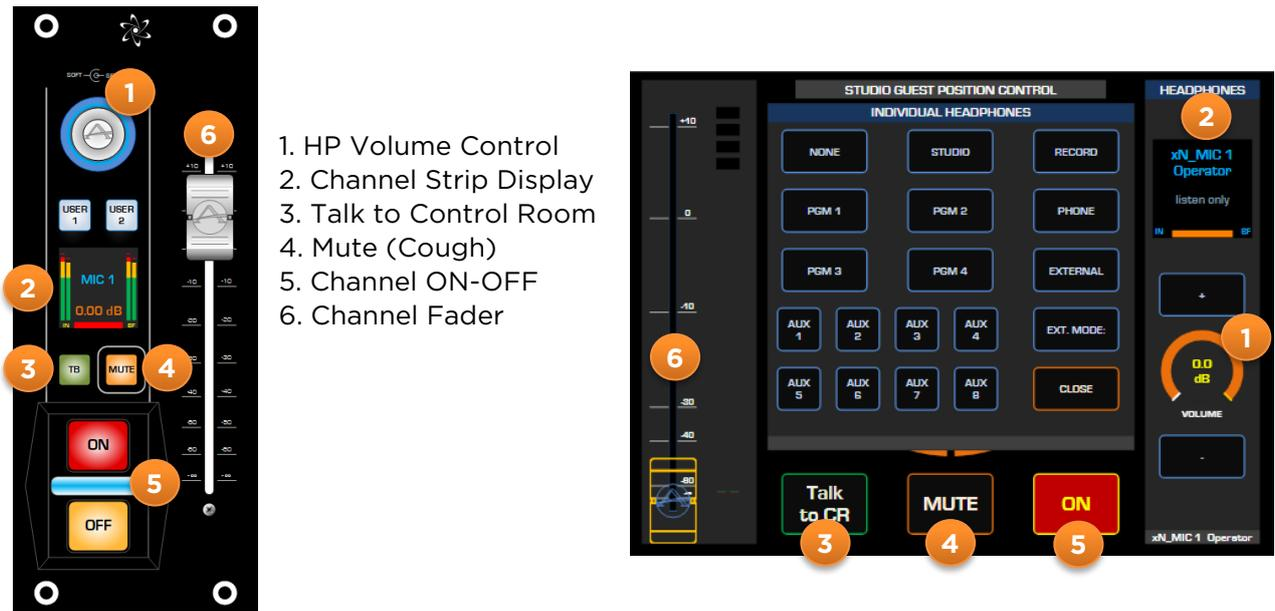
The large **+** and **-** buttons allow for fine adjustment of the headphone level in steps of 1dB while the Volume gauge allows for quick adjustment by swiping the control left or right.
