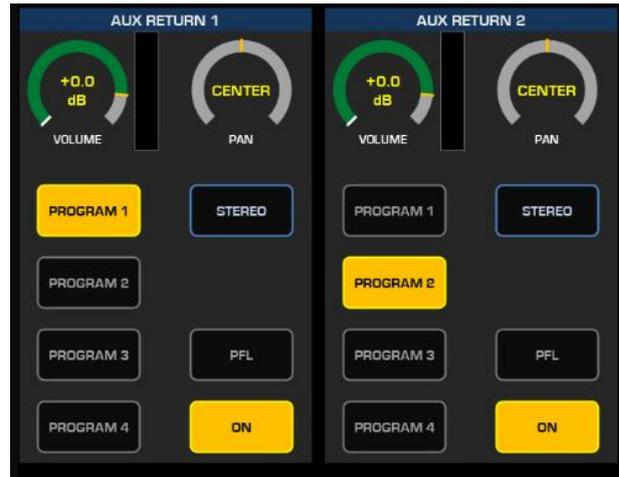
Additionally, the AUX returns can be monitored as part of PFL via the dedicated soft buttons that are provided in this view. The action of these buttons is always momentary.
