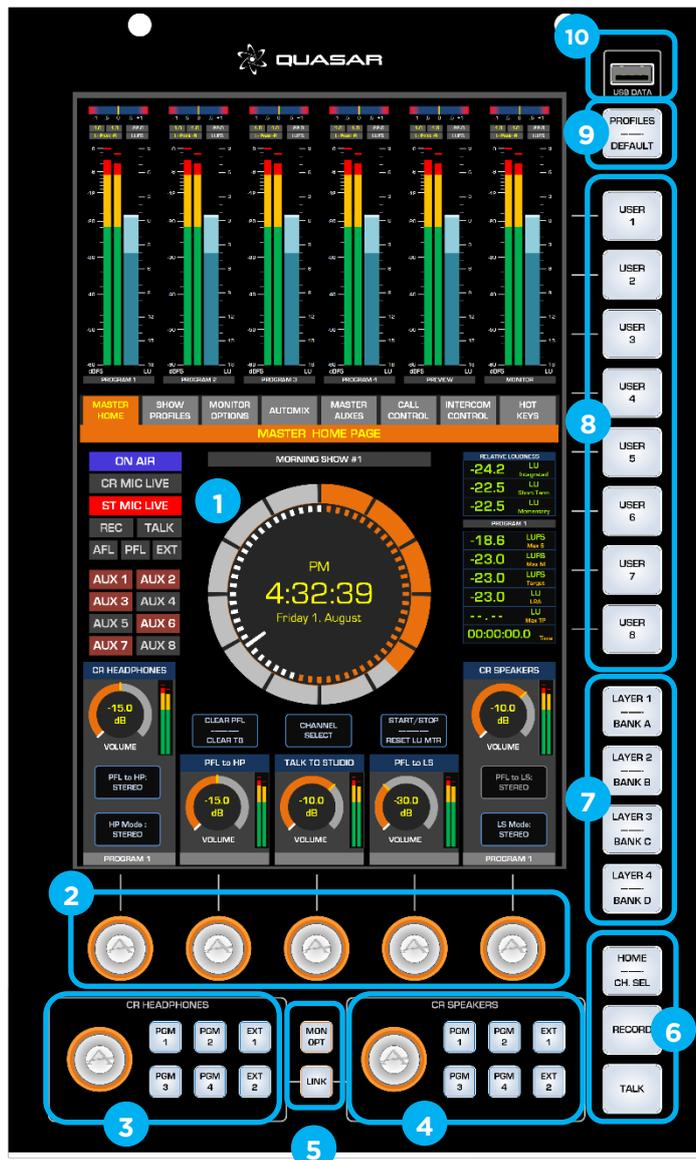
When the rotary encoder is touched, and a UI tab other than the MASTER HOME tab is selected in the UI, a small pop-up window will appear on the display (1), showing the Headphone Volume information.
