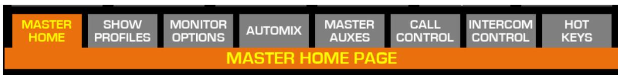
These are located always in the middle of each page, (for easy reach and to split the Main Meters area from the Controls area) and can be operated as buttons (although they don't look like a button widget) to access each of the GUI pages. The tab names and their order are fixed, not user-defined.
