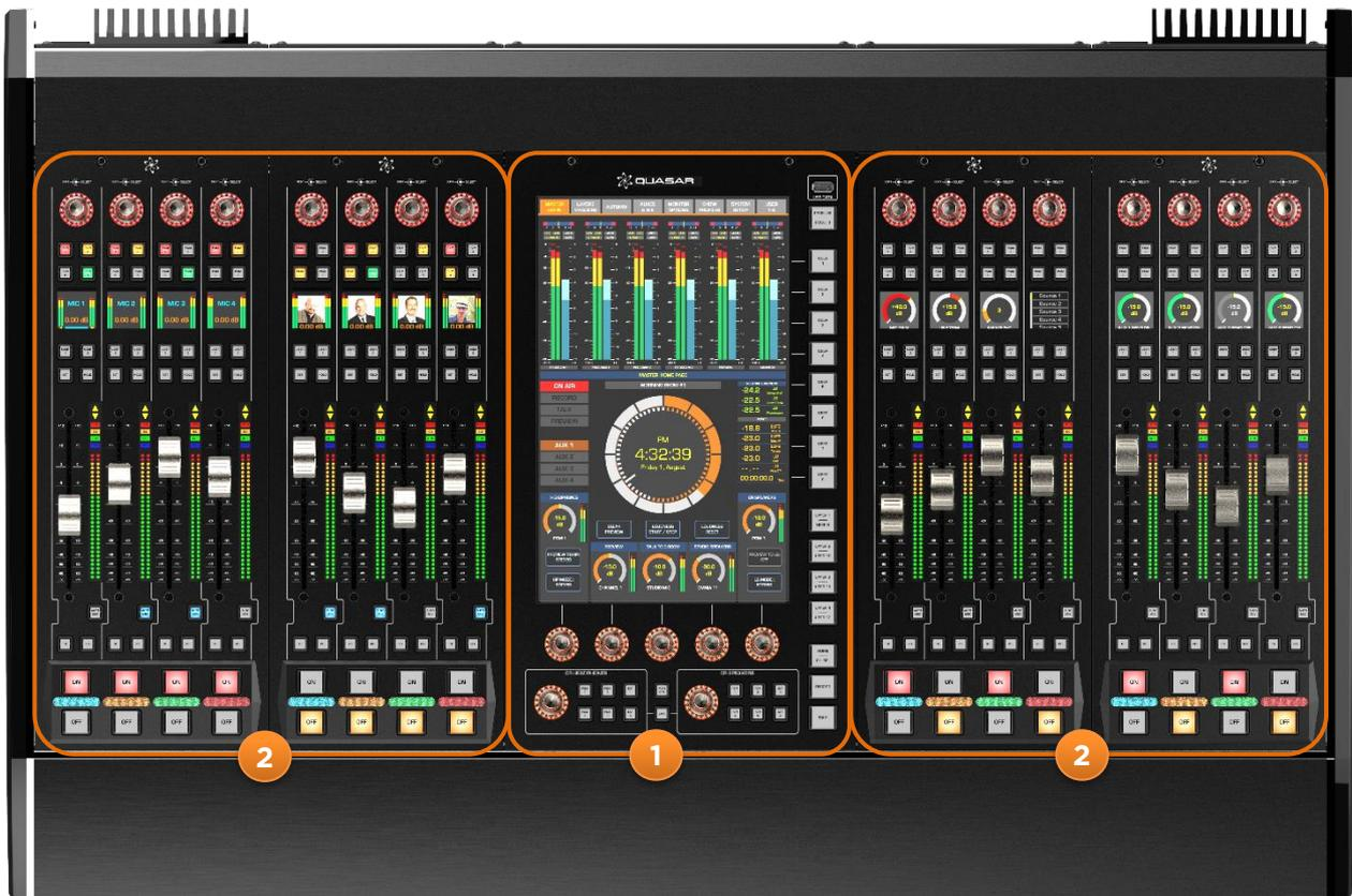
1. MTS-MON Module: Main Master and Monitor Control Module.
