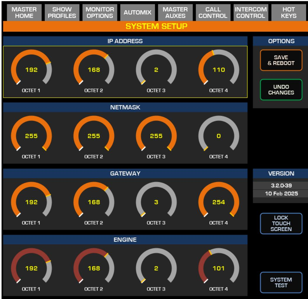
The IP ADDRESS, NETMASK, GATEWAY and ENGINE sections are for configuring the network parameters of the Console and Engine, without using their Web UIs.
