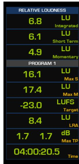
Below there are two Max True Peak values recorded for the Left and Right channels. Below the true peak meter is the time counter.
