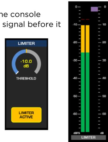
If the input level of the signal is such that very low thresholds are required, in order to see some gain reduction activity on the meter, we suggest adjusting the input gain or the previous channel processing stages to "beef up" the signal, maintaining the proper operating levels throughout the entire input channel.
