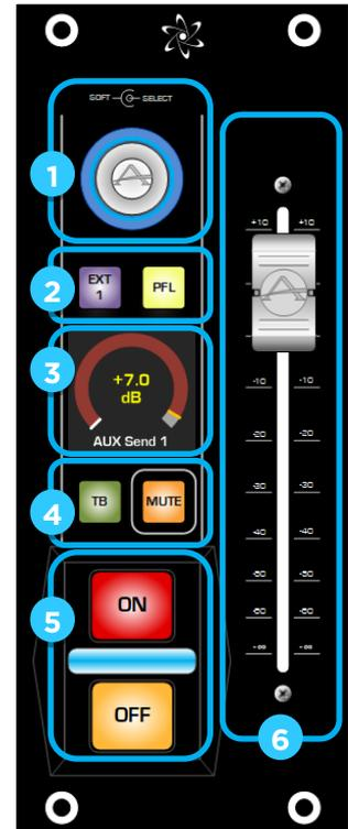
A full description of how to configure Accessory Modules for different Operating Modes is available in Configuration Chapter 1: [Web UI Reference: ACC Modules](#).
