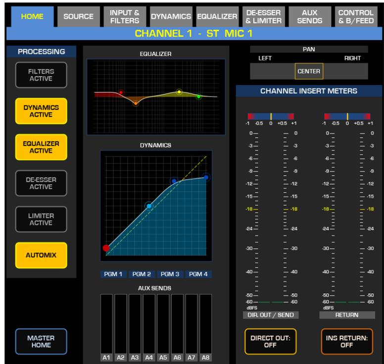
The Channel meters provide monitoring at-a-glance of the Direct Out (insert Send) and Insert Return levels. The EQUALIZER, DYNAMICS, and AUX SENDS graphs can be touched to go directly to the corresponding processing tab.
