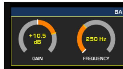
In addition to being operated from physical encoders, upon selection with a frame, Gauges can also be operated directly from the console touchscreen, by touching their area and swiping horizontally, (right to increase, left to decrease value) with your fingertips.
